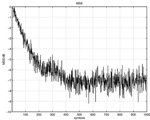
Figure 5. Learning curve for the serial receiver.
