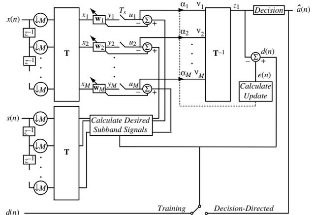
Figure 3. Parallel, adaptive DSSS receiver.
