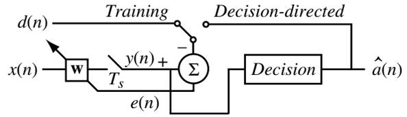
Figure 2. Fractionally-spaced adaptive DSSS receiver.
