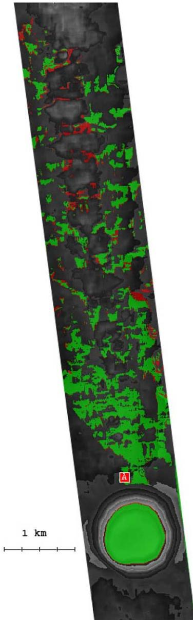
Fig. 8. Antenna coverage pattern for Gusev3, Site 2 (see Fig. 1). The red square with “A” indicates location of transmitter. Red areas denote 1 Mbps, green areas denote 11 Mbps. (For interpretation of the references in colour in this figure legend, the reader is referred to the web version of this article.)
