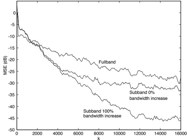
Figure 5: MSE for the subband adaptive filter systems with 0% and 100% analysis filter bandwidth increase and the fullband adaptive filter system under SIRP input.
