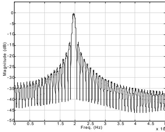
Fig. 3: Average DAMA power spectrum (Doppler-shifted and spread)
