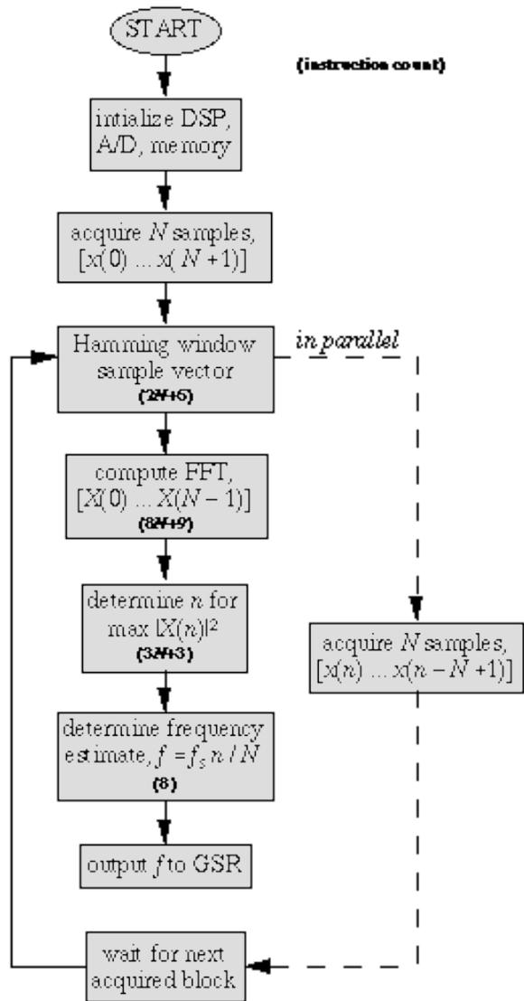
Figure 6: Flow diagram of Motorola DSP56303 software for frequency estimator
