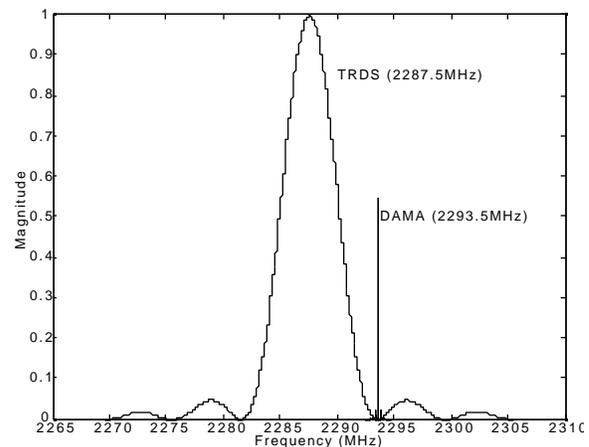
Fig. 1: Proposed spectral location of DAMA request.
