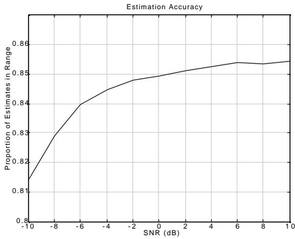
Fig. 5: Estimation accuracy for various SNRs
