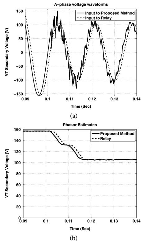
Fig. 4. Phasor estimation with a traditional relay and with the proposed approach for LGF at 100 km from the sending end.
