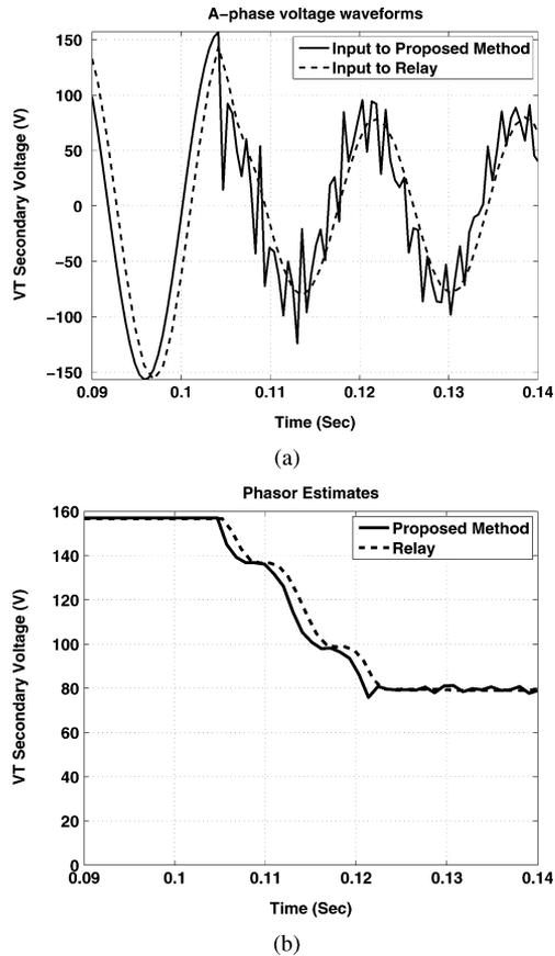
Fig. 2. Phasor estimation with a traditional relay and with the proposed approach for a sampling rate of 1.92 kHz.
