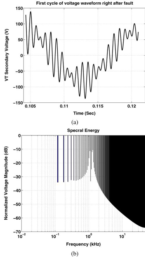
Fig. 1. Voltage waveform and its spectral energy using a sampling rate of 96 kHz.
