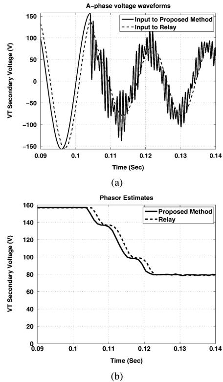
Fig. 3. Phasor estimation with a traditional relay and with the proposed approach for a sampling rate of 48 kHz.
