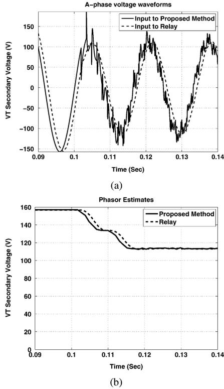
Fig. 5. Phasor estimation with a traditional relay and with the proposed approach for LLLF at 150 km from the sending end.
